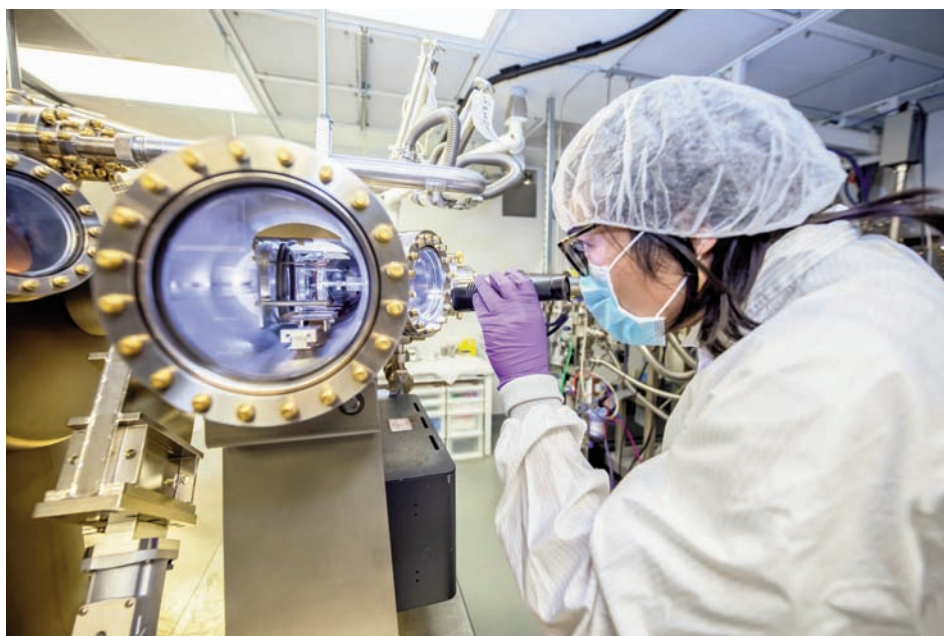
The experimental setup in Zetian Mi's lab where his team prepared an artificial photosynthesis device that can turn carbon dioxide and water into ethylene, in a step toward making solar fuels. Yuyang Pan shines a light on the device. Image credit: Sylvia Cardarelli and Jero Lopera, Electrical and Computer Engineering, University of Michigan
