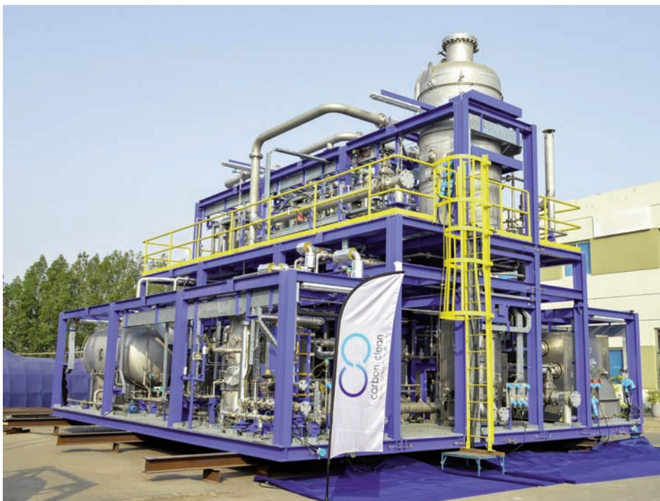
CycloneCC is a cost-effective, modular and compact carbon capture solution that is easy to scale
