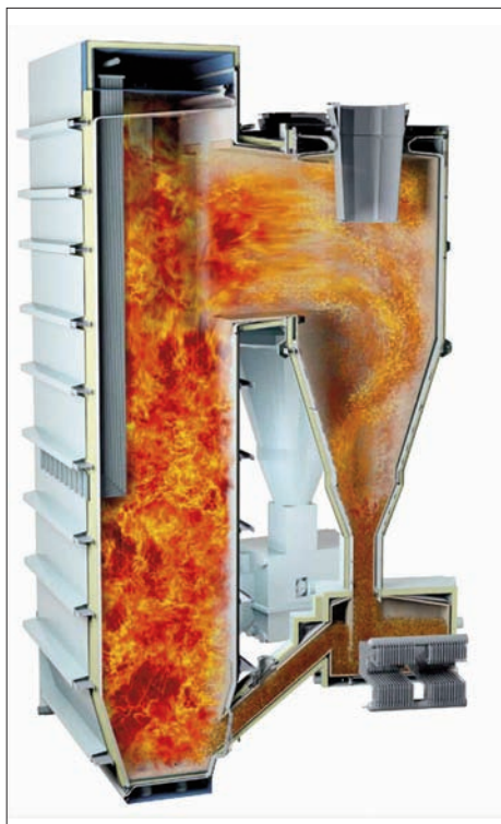
Fig. 2 - Circulating fluidized bed (CFB) boiler
