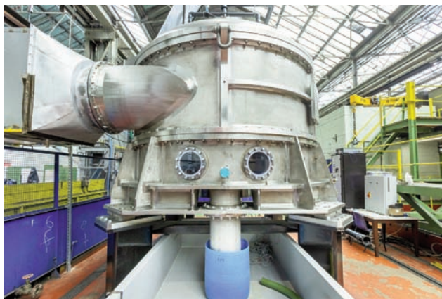
The CycloneCC C1 RPB represents a more than 20-fold RPB scale-up from the first industrial demonstration of CycloneCC, which was designed to capture up to 10 tonnes of CO 2 per day
