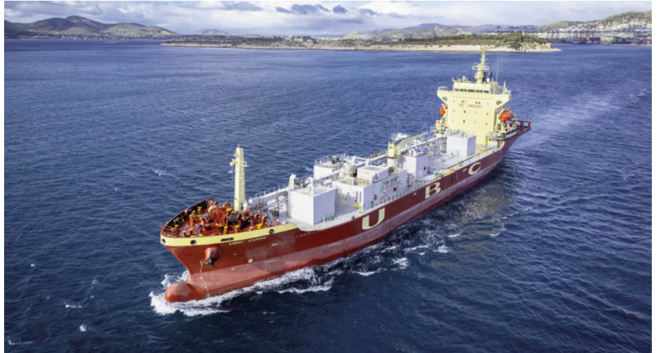
Seabound is deploying its compact marine carbon capture system aboard the UBC Cork (pictured). The captured carbon will be offloaded as limestone at the Port of Brevik, Norway, for use at Heidelberg Materials' nearby cement plant
