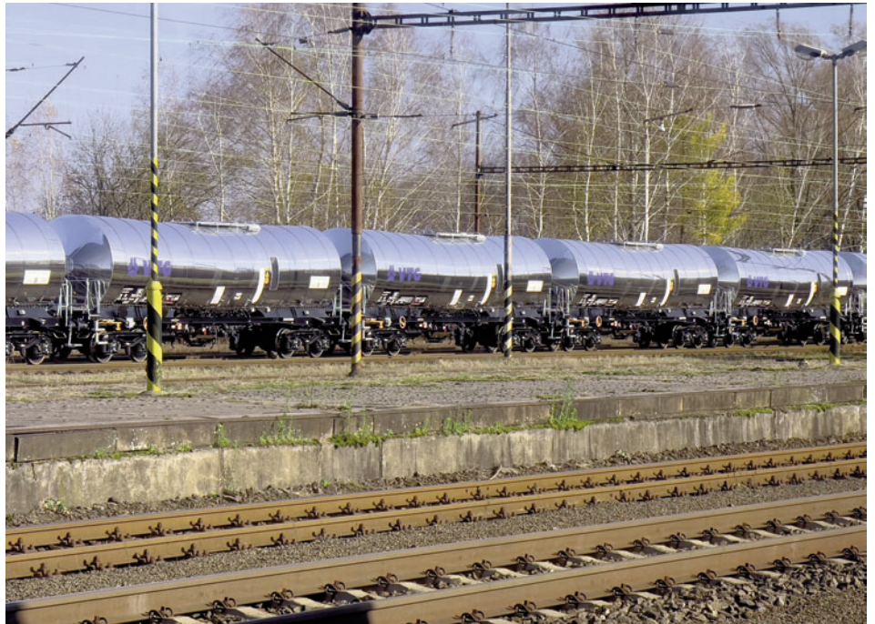
Bulk liquid movement by rail – a cement plant capturing 1 MT CO 2 per year would need one train per day with 30 waggons to transport liquefied CO 2
