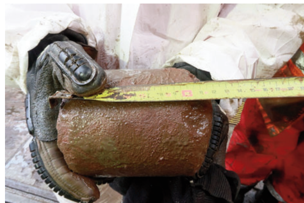
Core sample taken from well C43/30-2
