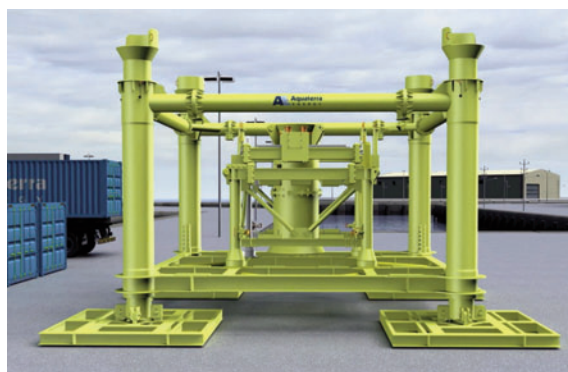
Aquaterra's Recoverable Abandonment Frame (RAF) system can reduce the time and costs of well abandonment
